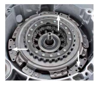
• Apply first puller leg between clutch housing and clutch and pull upward, simultaneously inserting the dowel on the underside into the hole in the puller leg.
