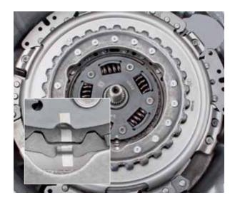
• Apply snap ring with the gap equally spaced around the large tooth.
