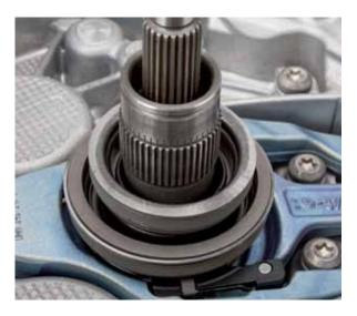
• Position reference gauge 32.92 mm (KL-0500-6032) on small engagement bearing (for K2).
