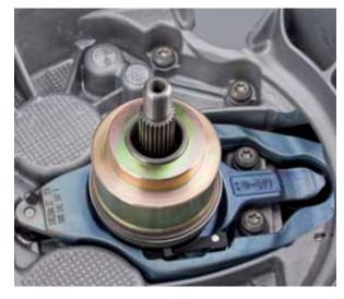
• Position 3.5 kg weight (KL-0500-6034) on reference gauge to generate specified preload.
