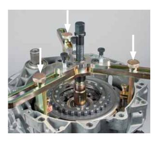
• Tighten three hexagon socket screws on the cross beam.
