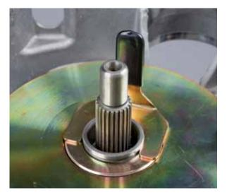
• To check whether or not correct adjusting shim is fitted, try to move engagement bearing reference gauge axially against setting gauge in position using corresponding engagement lever.
