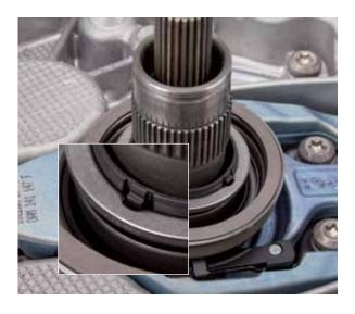
• Insert small engagement bearing (for K2) and ensure flanges fit properly in engagement bearing grooves.
