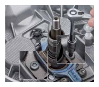
• Remove bracket, engagement lever and guide sleeve; bracket is missing on previous transmission designs.
