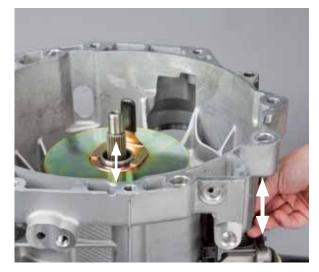
• Fine-tune adjusting shim corresponding to clutch nominal setting to individual tolerance values of clutch K1.
