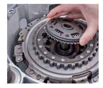
• Remove snap ring from hollow shaft by means of circlip pliers (KL-0192-12). Normally, ring gets damaged and needs to be replaced.
