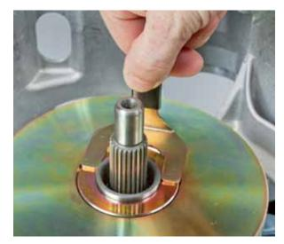
• Repeat until the adjustment gauge can be pushed into the retaining ring groove without force – the adjusting shim for the standard size of clutch 2 has been identified.
