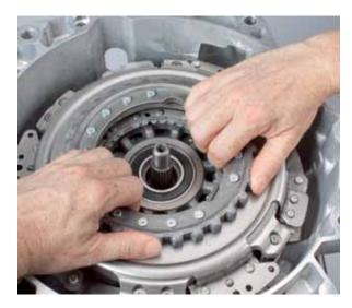
• Measure distance between top edge of bearing inner ring and frontal area of hollow shaft to ensure clutch fits properly on shaft. Distance must not exceed 8 mm.
