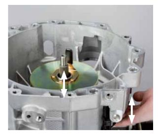
• Fine-tune adjusting shim corresponding to clutch nominal setting to individual tolerance values of clutch K2.
