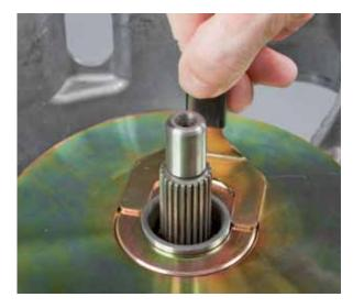
• Repeat until the adjustment gauge can be pushed into the retaining ring groove without force – the adjusting shim for the standard size of clutch 1 has been identified.
