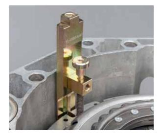
• Position support bush (KL-0500-6030) on hollow shaft.
