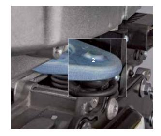
• Assemble thickest adjusting shim (2.8 mm) on big engagement bearing.
