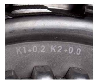
• Install calculated adjusting shim into big engagement bearing (for K1) and ensure it fits snugly in corresponding recess.
