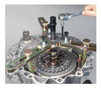
• Rotate spindle to remove clutch assembly from hollow shaft.
