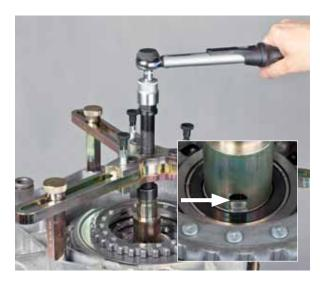
• Apply snap ring on hollow shaft using circlip pliers (KL-0192-12).
