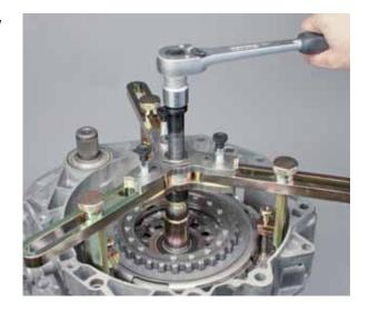
• Use cross beam to lift clutch assembly out of gearbox unit.
