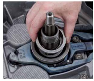
• Remove big engagement bearing (for K1), adjusting shim and engagement lever.
