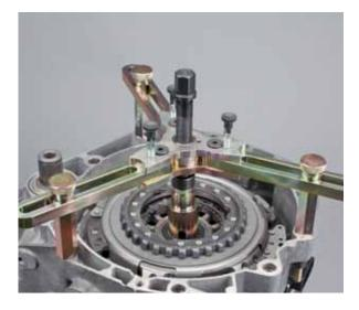
• Tighten three hexagon socket screws on the cross beam.
