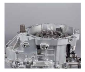
• Use screwdriver to remove snap ring of upper clutch disc hub (K1).
