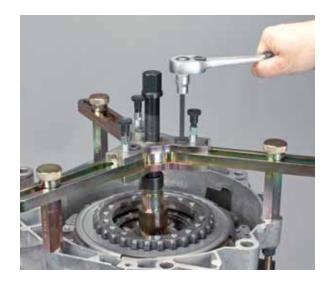
• Press the clutch on using the fitment tool onto the hollow shaft by tightening the spindle; The clutch is correctly fitted when the circlip groove is completely visible in the window of the fitment tool and the effort required to turn the spindle increases noticeably.
