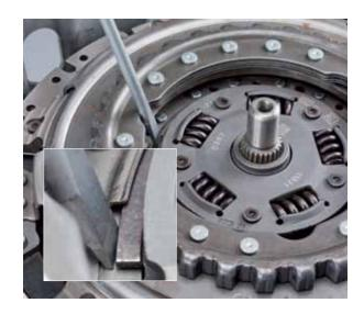
• Disassemble snap ring and clutch disc hub (K1).
