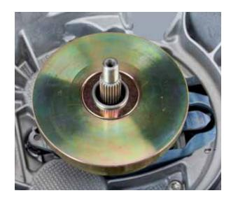
• Try to slide setting gauge (KL-0500-6035) into snap ring groove on hollow shaft.
