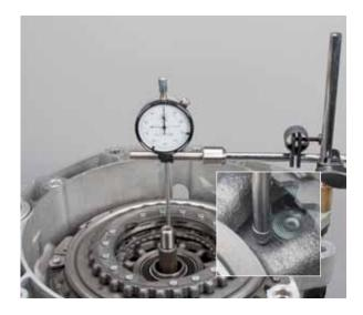
• Grab bottom clutch disc with two pull hooks, lift disc with both hands simultaneously until it contacts end stop and read off measurement.
