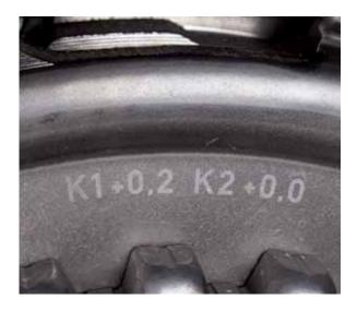
• Install calculated adjusting shim, mount engagement bearing (K2) and ensure flanges fit snugly in adjusting shim and engagement bearing grooves.
