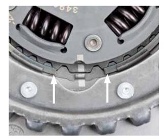
• Measure end float of top clutch disc (K1). Position preloaded measuring tip on top clutch disc hub and zero the dial gauge.
