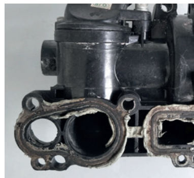
Fig. 5: Leakage due to additional sealant (damage symptoms)
