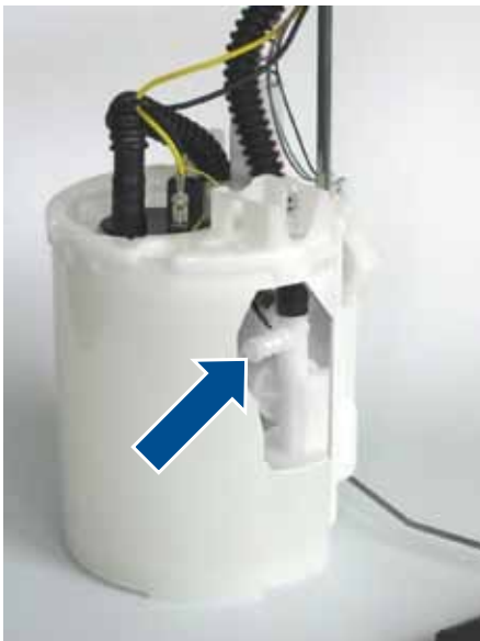
Fig. 1: View into the fuel delivery module (elevation) with blind-mate connector
