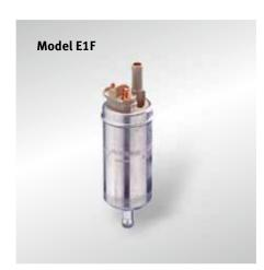
A frequently used pump is the model E1F. This is an in-line positive displacement pump with a sliding vane pumping stage and it is suited for system pressures of 0.1 to 1.0 bar.
