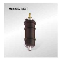
Model E2T / E3T fuel pumps are self-priming toothed ring pumps and have been designed to handle higher flow rates. Located on the delivery side is a pressure holding valve, which depending on the model of the pump is either integrated within the pump or is accommodated in exchangeable screw-in fittings. An integrated pressure limiting valve
