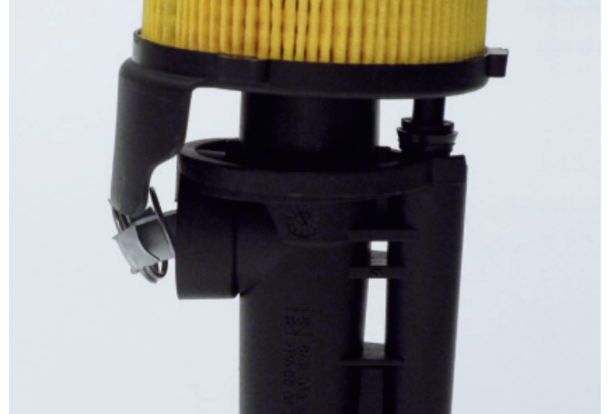
Figure 4: Detailed view of the damaged by-pass valve.
